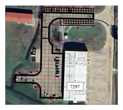
There will be two different pavement sections, one will be for vehicle parking and non-trailer use and the other for MHU 96 towing trailer use.
