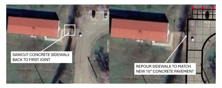
The contractor will not bury any chunks of concrete. Any concrete chunks can be delivered to our concrete rubble stockpile within one mile of the job site.
